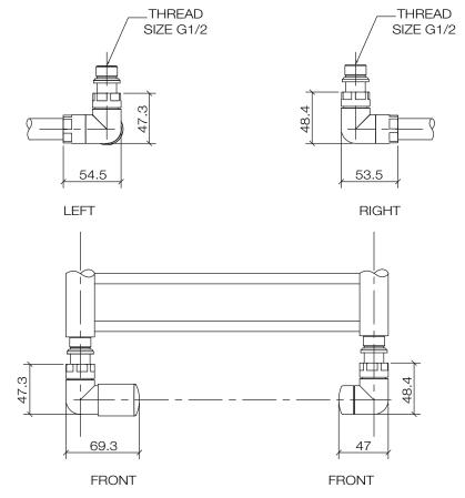
Pipe fixing centers = towel rail pipe centerlines
